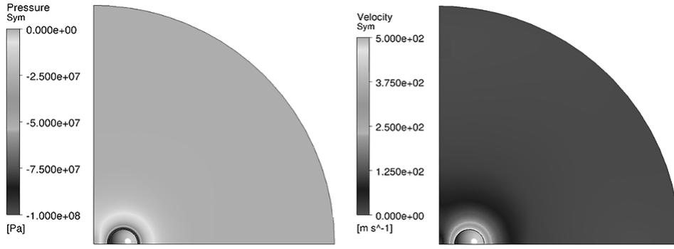
**Fig. 4** CFD simulations showing the velocity field (on the right) causally associated with the pressure gradient around a vortex-particle attracting the DS. From it we can have an absorption velocity  $v_a$  in any point of the field.
