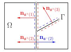
Figure 1: Example of a 2D domain  $\Omega$  and 3 intersecting fractures  $\Gamma_i$ , i = 1, 2, 3. We define the fracture plane orientations by  $\mathfrak{a}^{\pm}(i) \in \chi$  for  $\Gamma_i$ ,  $i \in I$ .
