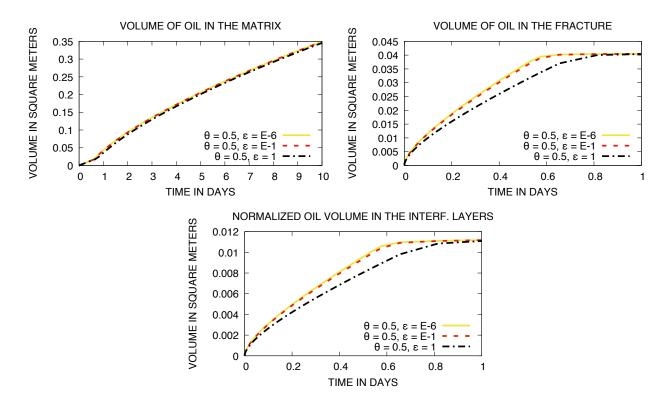
Figure 6: Volume occupied by oil in the matrix, fracture and oil volume normalised by  $\varepsilon$  in the interfacial layers, for  $\theta = 0.5$ , as a function of time.
