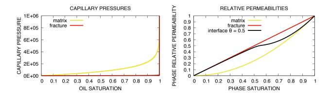
Figure 4: Curves for capillary pressures and relative permeabilities.
