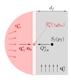
Figure 2: Illustration of the coupling condition. It can be seen as an upwind two point approximation of  $Q_{f,\mathfrak{a}}^{\alpha}$ . The upwinding takes into account the damaged rock type at the matrix-fracture interfaces. The arrows show the positive orientation of the normal fluxes  $\mathbf{q}_m^{\alpha} \cdot \mathbf{n}_{\mathfrak{a}}$  and  $Q_{f,\mathfrak{a}}^{\alpha}$ .
