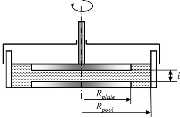
Fig. 3. Sketch of the experimental pool geometry
