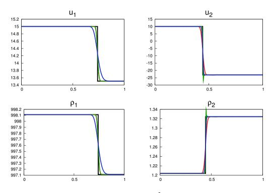
Figure 4: Approximate solution for test case 1 at  $T = 16.10^{-5}$  s. with 1000 cells. - Exact solution, -  $SP_m$ , -  $SP_a$ , - Rusanov.
