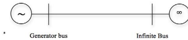
Figure .5: SMIB test system: generator connected to an infinite bus
