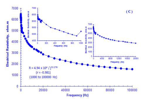
Fig. 1. Electrical signature, electrical resistivity *versus* AC frequency, for the studied Fe-Ni models: (A) 9.7% Ni, (B) 17.5% Ni, and (C) 30.0% Ni.
