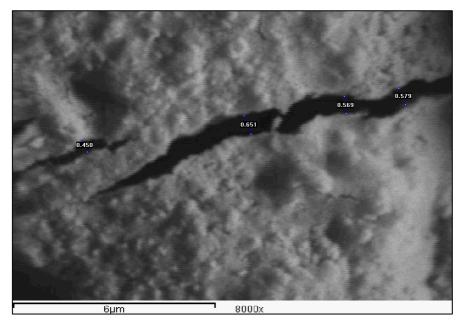
Fig. 6. SEM photomicrograph indicates the presence of some micro fractures of wideness not more than  $0.65 \mu m$ , NWA 869 sample.
