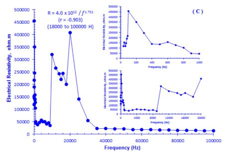
Fig. 3. Electrical resistivity *versus* AC frequency "electrical signature" for the studied stony meteorites: (A) NWA 869, (B) NWA 7629, and (C) Ghubara meteorite.
