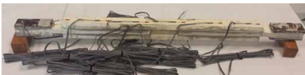
Figure 8. Joint sample “II” (after strain gauges application).
