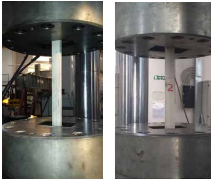
Figure 5. Preliminary tests on GFRP samples: Sample "1" (left) and Sample "2" (right).
