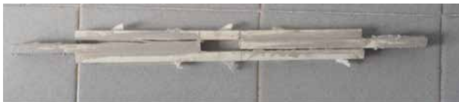
Figure 15. Post-failure configuration—joint sample “II”.
