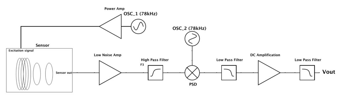
A high pass filter, will act to remove the low frequency signals and the bias on the output of the amplifier stage. Afterward a multiplier which is also known as the phase sensitive detector (PSD) or mixer, multiply the output of the AC amplifier by the external reference signal. By feeding the PSD output into a low pass filter the AC part of the signal is strongly attenuated. Thus, the output of the lock-in amplifier can be expressed as:
