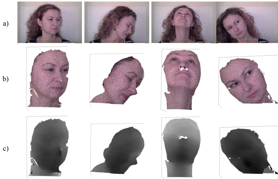
Fig. 6. Four frames from a movie of a moving female face. 3D reconstruction was performed using the pseudorandom dots pattern. Rows contain: a) input frames; b) textured 3D surface where input image is used as texture; c) 3D surface textured as depth map.
