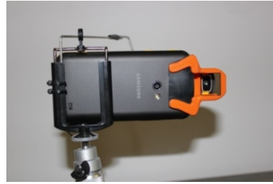
Fig. 2. Smartphone on a tripod with the deflection adapter for projector attached. Note the mirror image of the projector, i.e. a virtual projector.
