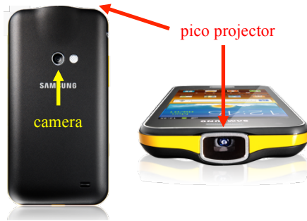
Fig. 1. Samsung Galaxy Beam: a camera and an embedded pico projector comprise an angle of 90^\circ , having no common FOV.
