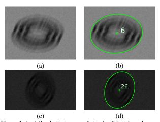
Figure 1. (a,c) Synthetic images of circular fiducials under very challenging shooting conditions *i.e.*, perturbed, in particular, by a (unidirectional) motion blur of magnitude 15px. (b,d) Using the proposed fiducial system, markers are correctly detected and identified with an accuracy of 0.54px and 0.36px resp. in (a) and (c) for the estimated imaged center of the outer ellipse whose semi-major axis (in green) is equal to 31.9px and 34.5px resp.
