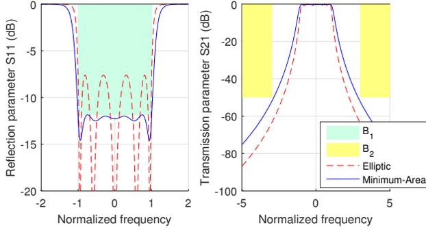
Fig. 2. Example of filter responses satisfying the constraints.
