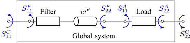
Fig. 1. Global system structure and scattering parameters.
