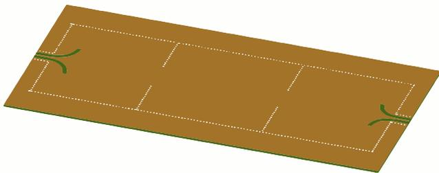
Fig. 4. Structure of the 3-poles *substrate-integrated-waveguide* (SIW) filter fed with *coplanar-waveguide* (CPWG) transmission lines designed with the software *Ansoft Electronic Desktop* and featuring a footprint of 120x40 mm.
