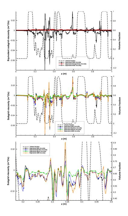
Figure 7: Comparison of equivalent turbulent viscosities obtained with DNS and LES MFA models, *i.e.* Smagorinsky [5], WALE [6], Bardina [7], Mixed model [8] and ADM [9]. The bottom line is a zoom on the middle plot. The results are plotted in a vertical line centered on [x = 0.8, y = 0.8]. The volume fraction is also plotted to locate interface position as C = 0.5.
