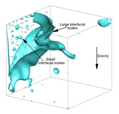
Figure 1: Example of multi-scale interfacial character of phase separation for a liquid-liquid two-phase system. The interface is plotted in blue and the black lines represent the wall of the cubic box. Following [2,3,15], Re=7000 and We=11.
