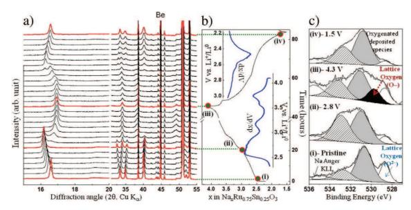
Fig. 4. Characterization of Na<sub>2</sub>Ru<sub>0.75</sub>Sn<sub>0.25</sub>O<sub>3</sub> sample a) insitu XRD patterns; b) voltage profile; and c) O1s XPS spectra.
