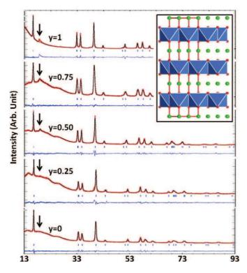
Fig. 1. XRD patterns for the  $Na_2Ru_{1-y}Sn_yO_3$  solid solution. Inset shows a projection of the layered structure.
