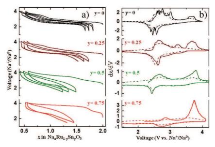
**Fig. 2.** Na<sub>2</sub>Ru<sub>1- $\nu$ </sub>Sn<sub> $\nu$ </sub>O<sub>3</sub> electrochemical behavior a) voltage composition curve and b) derivative plots.
