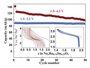
Fig. 3. Cycling behavior of the Na<sub>2</sub>Ru<sub>0.75</sub>Sn<sub>0.25</sub>O<sub>3</sub> sample.
