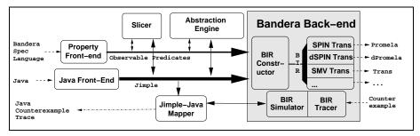
Figure 1. Internal architecture of the Bandera Tool Set
