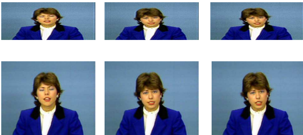
Figure 7: Claire sequence: degraded low resolution fields (top), restored high resolution images (bottom).
