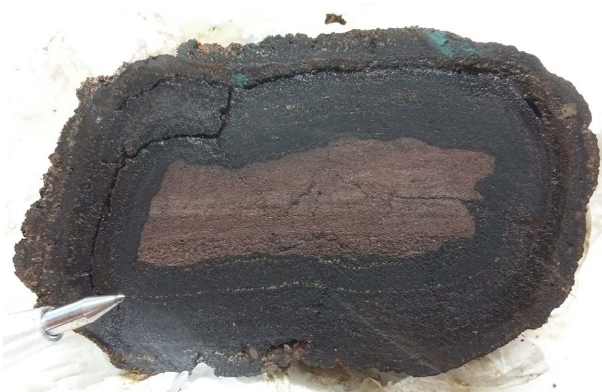
Figure 58: Sedimentary clast (claystone) in a nodule (DRA-E1-8).
