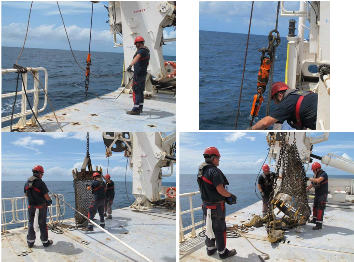
Figure 9: Operations to bring back the dredge A1 on deck. From left to right and up to down: 1- the dredge hangs below the swivel (red) and the Grand Fond cable; the cable of the working winch is attached to the shackle below the swivel. 2- the dredge hangs on the working winch, the GF cable and the swivel are going to be removed. 3- the dredge is on deck, and then 4- turned upside-down to be emptied.
