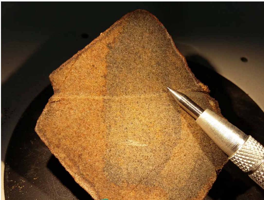
Figure 25: Section of sample DRA-G2-2: fine sandstone.
