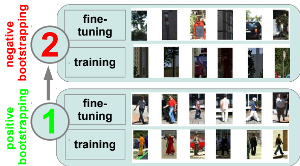
Fig. 2: Temporal sequence of training steps during the bootstrapping process from a source dataset (usually synthetic) to a target dataset (usually real-world, here: KITTI). The first step of positive bootstrapping includes training on positive samples from the source dataset, then training on positive samples from the target dataset. The subsequent negative bootstrapping is conducted in an analogous fashion except that it excludes "easy" negative samples.
