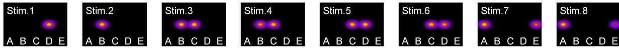
Fig. 6. The eight 100x100 pixel test stimuli used in the experiments, consisting of superpositions of Gaussians (axes are scaled differently). Gaussian amplitudes are 1.0 where not otherwise stated. In stimulus 4, the Gaussian at site B has amplitude 0.9. In stimulus 6, the Gaussian at site D has amplitude 0.8. In stimulus 8, the Gaussian at site D has amplitude 0.5.
