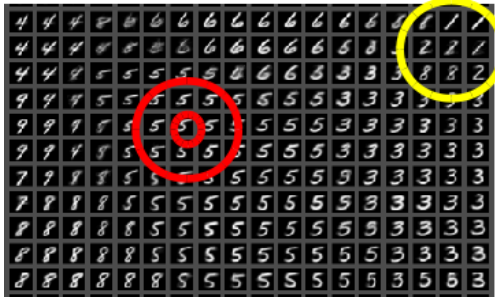
Figure 3. Illustration of how incremental learning is made possible through a topologically ordered prototype representation. Due to topological ordering, neighbouring prototypes are almost always situated in nearby regions of input space. Therefore, local updates of prototypes will almost always be local in input space as well, thus effectively enabling efficient incremental learning. This is shown here for a subset of prototypes trained on the MNIST database, the best-matching unit (BMU) for a "5" input being indicated by a small red circle. It is obvious that the local 2D update region, indicated by a larger red circle, is indeed local in the input space. The yellow circle indicates a region where this property does not hold (structural defect) but the reader can convince himself that this occurs but rarely.
