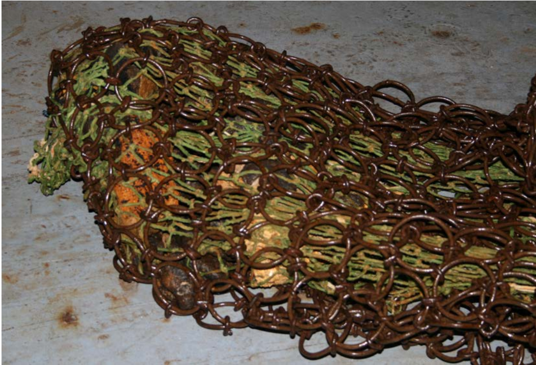
Figure 7: The two nets (inside in nylon, outside metallic) on the deck at the end of dredge E1.
