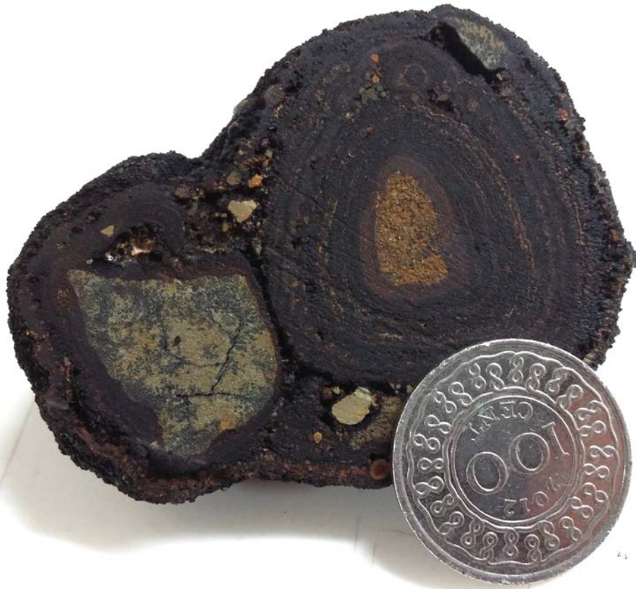
Figure 24: Section of sample DRA-G2-9. This nodule formed by encrusting two nodules together with several small fragments. The clast in the nodule on the right side is fine sandstone, the clast on the left side is a claystone.
