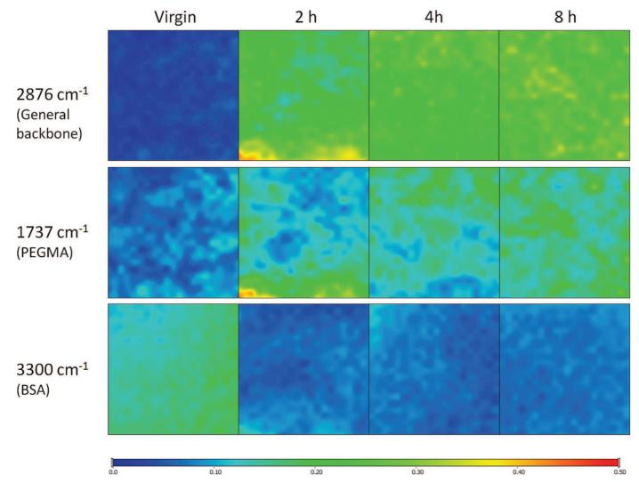
**Fig. 13.** Example of FTIR maps obtained for membranes modified with the random copolymer at different coating times while keeping the copolymer concentration at 5 mg/mL. Each map has an area of 1 mm<sup>2</sup>. (For interpretation of the references to colour in this figure legend, the reader is referred to the web version of this article).
