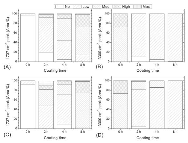
Fig. 14. Measured area percentages for the different coverage and adsorption levels as a function of coating time, for a 5 mg/mL copolymer solution. (A) and (B): Random copolymer; (C) and (D): diblock copolymer.
