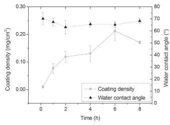
**Fig. 12.** Water contact angle and average coating densities as a function of coating time. Coating solution: 5 mg of random copolymer per mL of ethanol.
