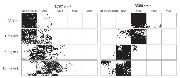
Fig. 9. Coverage and adsorption levels for the membranes modified with different random copolymer concentrations and a coating time of 2 h.
