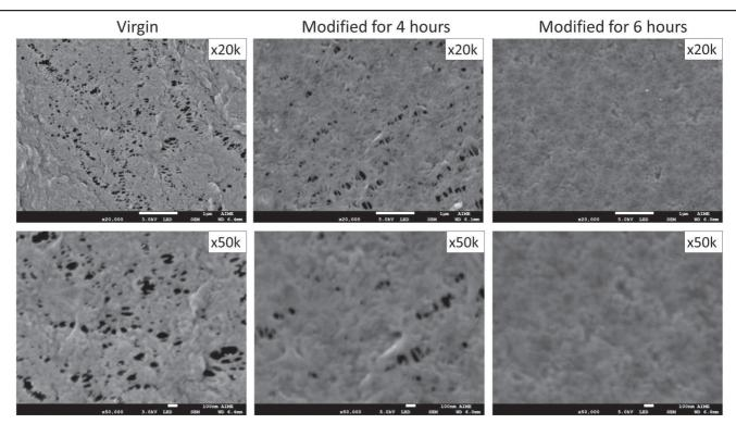
**Fig. 16.** SEM images of the virgin, and modified membranes: for 4 and 6 h, with a 5 mg/mL PS-r-PEGMA copolymer. The scale bars correspond to 1 μm and 100 nm for the × 20k and the × 50k magnifications, respectively. The images were taken with a Schottky Field Emission Scanning Electron Microscope (JEOL SEM-FEG JSM7800F); samples were metallised with gold.
