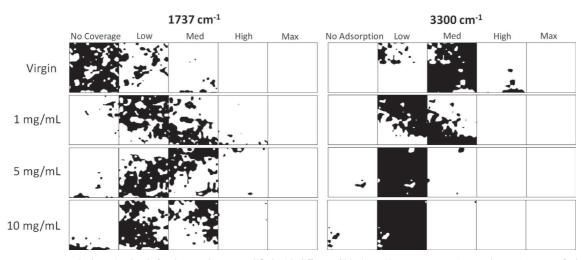
Fig. 10. Coverage and adsorption levels for the membranes modified with different diblock copolymer concentrations and a coating time of 2 h.
