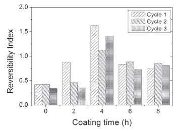
Fig. 17. Reversibility index calculated for the different membranes.
