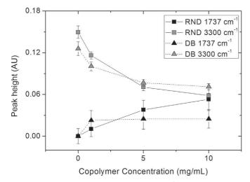
Fig. 7. Average peak height of the 1737 and  $3300 \text{ cm}^{-1}$  peaks as a function of random (RND) and diblock (DB) copolymer concentration.
