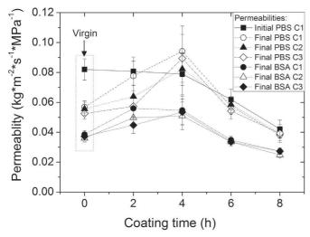
Fig. 15. Permeability as a function of coating time for the membranes modified with 5 mg/mL of copolymer solution.
