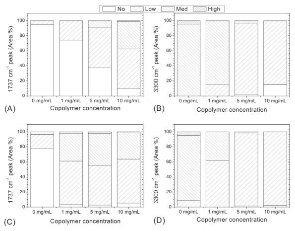
Fig. 11. Measured area percentages for the different coverage and adsorption levels as a function of copolymer concentration. (A) and (B): random copolymer; (C) and (D): diblock copolymer.
