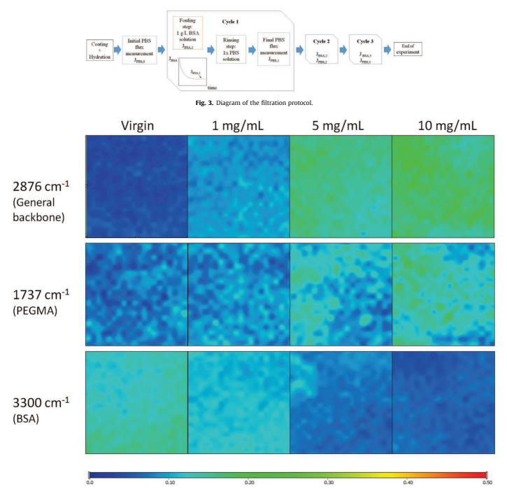
Fig. 4. Example of FTIR maps obtained for membranes modified with the random copolymer at different concentrations. Each map has an area of 1 mm<sup>2</sup>.
