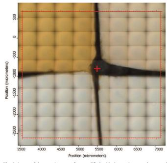
**Fig. 6.** Image of the membrane surface modified with the random copolymer and incubated with 1 g/L BSA solution. Virgin membrane (upper left) and modified with copolymer solution concentration of 1 mg/mL (upper right), 5 mg/mL (lower right), and 10 mg/mL (lower left). The mesh is a consequence of the images taken by the microscope to determine the subsequent surface to be analysed by the FTIR microspectrometer.
