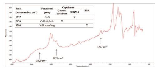
Fig. 1. Sample spectra of a coated and fouled membrane with additional information on the Peaks of interest, functional groups related to them and to the compounds present in our study.
