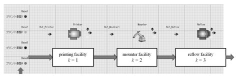
Fig. 2. Simulation model of the middle-scale semiconductor manufacturing line.
