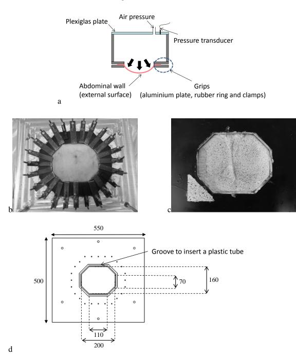
Figure 1. a) Scheme of the custom test apparatus. b) View of the grips exposing the external surface (prior to the application of the speckle) with aluminium plate, rubber ring and clamps
