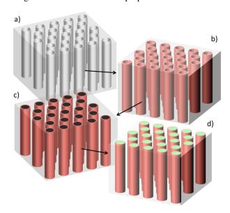
Figure. 1. (Color online) Schematics for the synthesis of the CFO-PZT NC arrays: a) porous AAO template, b) wet chemical deposition and cryztallisation of the PZT shells on the AAO pore walls, c) electrodeposition of the CF cores within the PZT-coated AAO pores, and d) CF conversion into CFO by *in-situ* thermal oxydation.
