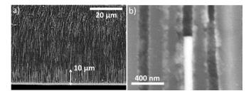
Figure. 4. (a) HRSEM fracture image of a CF-PZT<sup>700</sup> nanocable array embedded in the AAO template (150 nm pore diameter, 15% porosity). (b) Corresponding closed-up magnification of a single NC highlighting the three-phased AAO-PZT-CF morphology.
