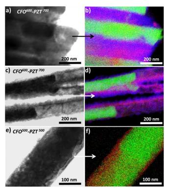
Figure. 7. (Color online) (a) STEM-BF micrograph of the CFO<sup>600</sup>-PZT<sup>700</sup> core/shell architecture within the AAO template after grinding and dispersion in ethanol. (c) The same sample after AAO etching in 1 M NaOH and dispersion in ethanol. (e) The CFO<sup>500</sup>-PZT<sup>500</sup> system after template etching and dispersion in ethanol. (b, d, f) Corresponding chemical mapping, with Pb, Fe and Al represented in red, green and blue, respectively.
