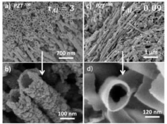
Figure. 2. HRSEM micrographs showing bundles of PZT<sup>700</sup> (a) and PZT<sup>500</sup> (c) tubular structures after the AAO template removal. (b, d) Corresponding higher magnification images. The pronounced granular aspect of the PZT<sup>700</sup> structures can be observed in panel (b).
