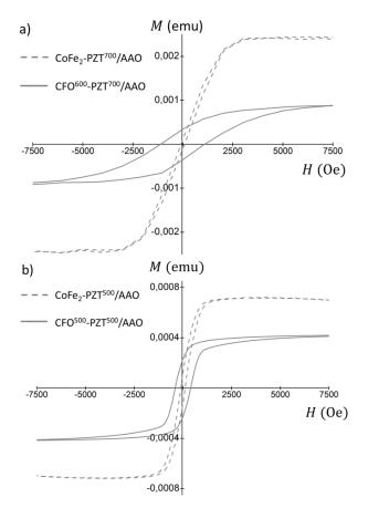
Figure. 9. (Color online) a) Room temperature hysteresis loops measured with the external field applied along the revolution axis of the CF-PZT<sup>700</sup> NCs (dashed line) and CFO<sup>600</sup>-PZT<sup>700</sup> NCs (solid line) embedded in AAO templates, b) the same as in a) for CF-PZT<sup>500</sup> NCs (dashed line) and CFO<sup>500</sup>-PZT<sup>500</sup> NCs (solid line)
