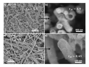
Figure. 6. (a, b) HRSEM micrographs at different magnifications, showing the dense arrays of CFO  $^{600}$ -PZT  $^{700}$  NCs after the AAO template etching in 1 M NaOH. (c, d) Micrographs at different magnifications acquired from the CFO  $^{500}$ -PZT  $^{500}$  NCs prepared in similar conditions.
