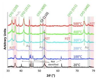
Figure. 8. (Color online) CF to CFO *in-situ* oxidation inside PZT followed by *in-situ* X-ray diffraction at different temperatures with an increment of 100°C. The starting room temperature CF pattern is represented in black and the final CFO oxidized one is in red.
