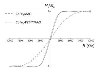
Figure. 5. Room temperature hysteresis loops measured with the external field applied along the revolution axis of the AAO-embedded CF nanowires (dashed line) and CF-PZT<sup>700</sup> NCs (solid line).
