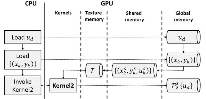
Figure 10: Software structure for the computation of complex waves scattered by point-source layers
