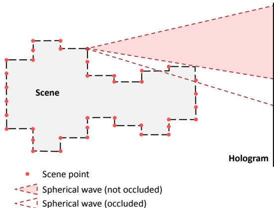
Figure 1: Light shielding using the point-source approach: a visibility test is done to check the existence of obstacles between an object point and each sampling point in the hologram plane.
