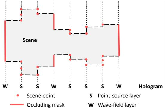
Figure 4: Hologram computation using the proposed hybrid approach.
