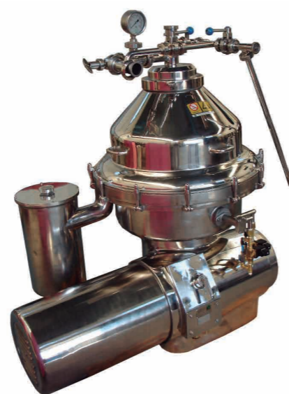
Hipercentrifugation on Alfa Laval MRPX-214
