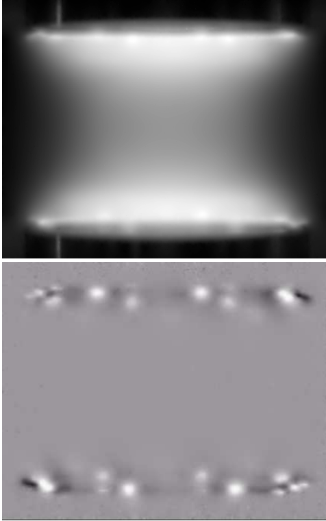
Figure 1. Rotating plasmoids during DPGI. Eight plasmoids in front of each electrode are moving with a clockwise rotation. Raw image and the filtered one after background subtraction. The background is obtained by averaging plasma emission over time (at least during a complete plasmoid rotation).
