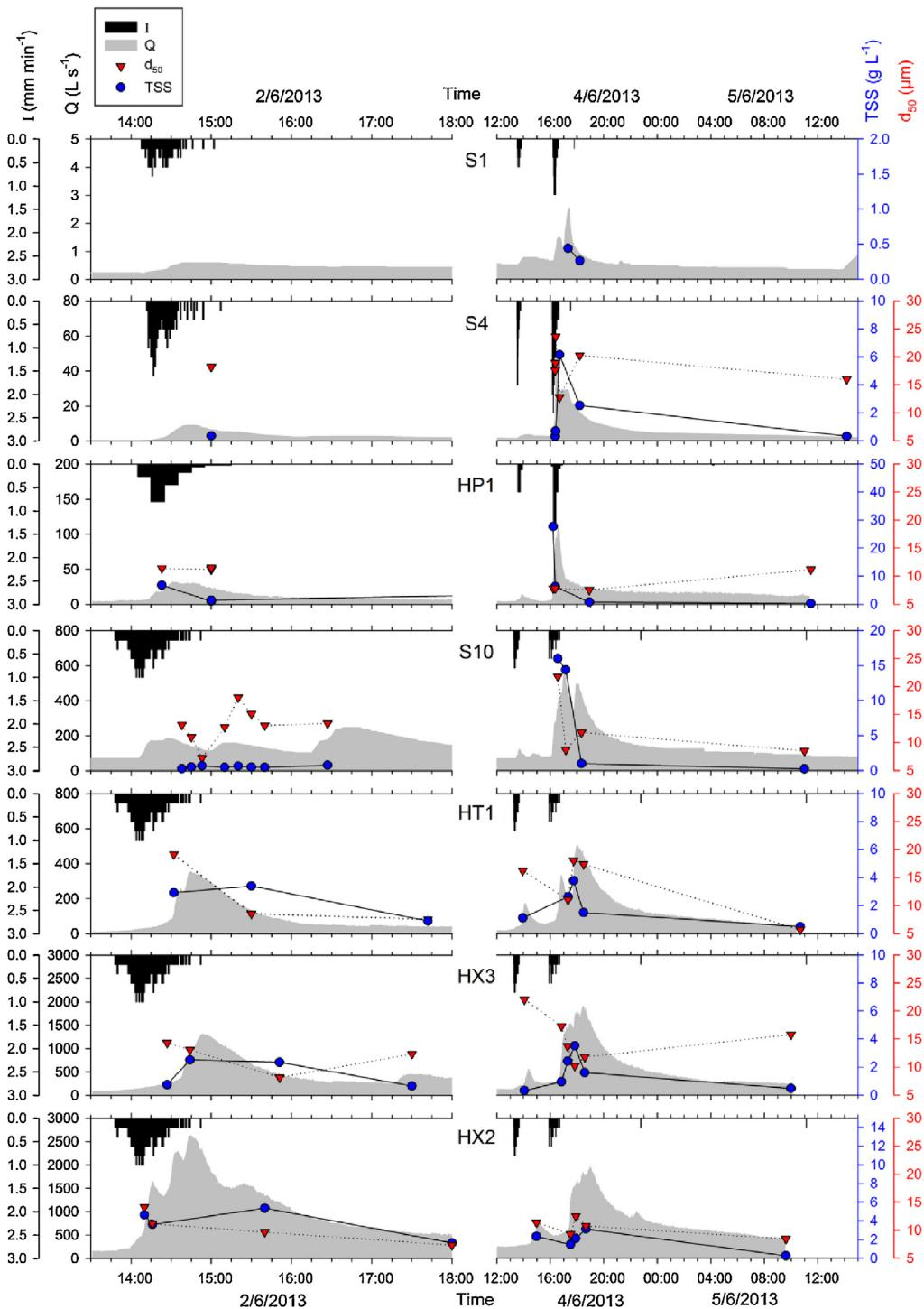
**Fig. 5.** Total suspended sediment loads (TSS, filled circles) and particle size distributions ( $d_{50}$ , triangles) during the June 2 and 4 floods at each station (location in Fig. 1). Shaded areas represent water discharge (Q), vertical bars rainfall intensity (I) at each station, except at HT1, HX3 and HX2 where rainfall data recorded at S10 were used. Note the different Q and TSS scales in each plot and the different time scales for each flood.
