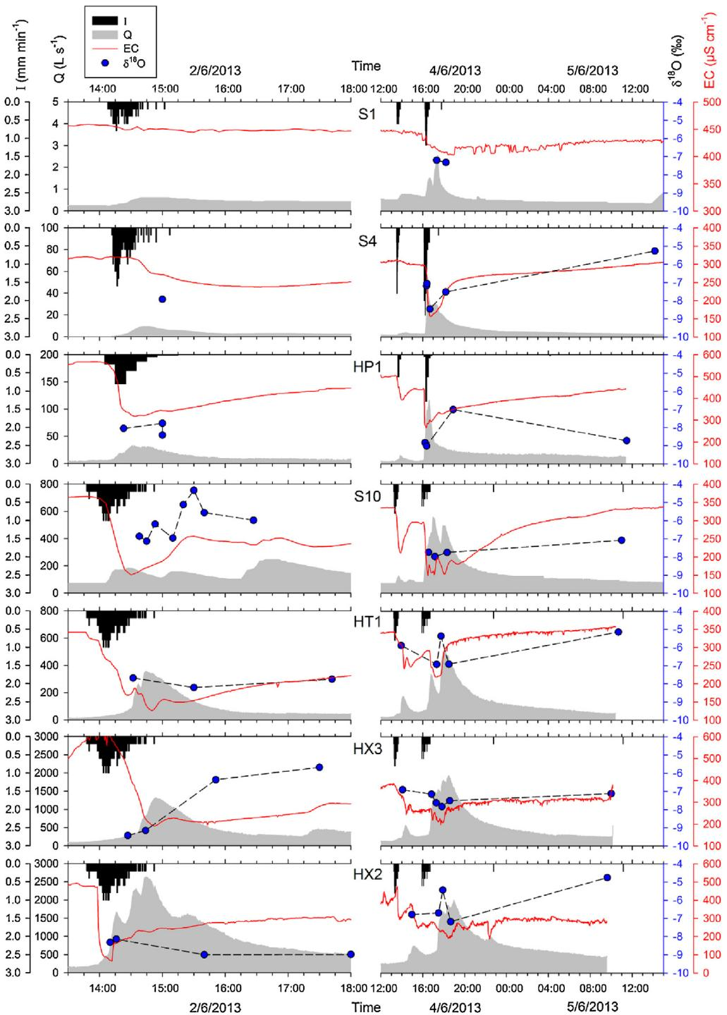
**Fig. 4.** Stream water  $\delta^{18}\text{O}$  (filled circles and dashed line) and water electric conductivity (EC, solid line) records during the June 2 and 4 floods at each station (location in Fig. 1). Shaded areas represent water discharge ( $Q$ ), vertical bars rainfall intensity ( $I$ ) at each station, except at HT1, HX3 and HX2, where the rainfall data recorded at S10 were used. Note the different  $Q$  and EC scales in each plot and the different time scales for each flood.
