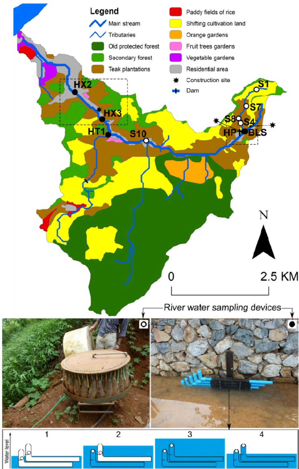
**Fig. 2.** Land use map of the catchment in 2012 and river water sampling devices installed at the different stations. Left picture: automatic pumping sampler; right picture: passive auto-capping collector (flood rise sampling). Bottom sketch: section views of the sampling stages of the passive auto-capping collector during water level rise (1–3) and decrease (4).
