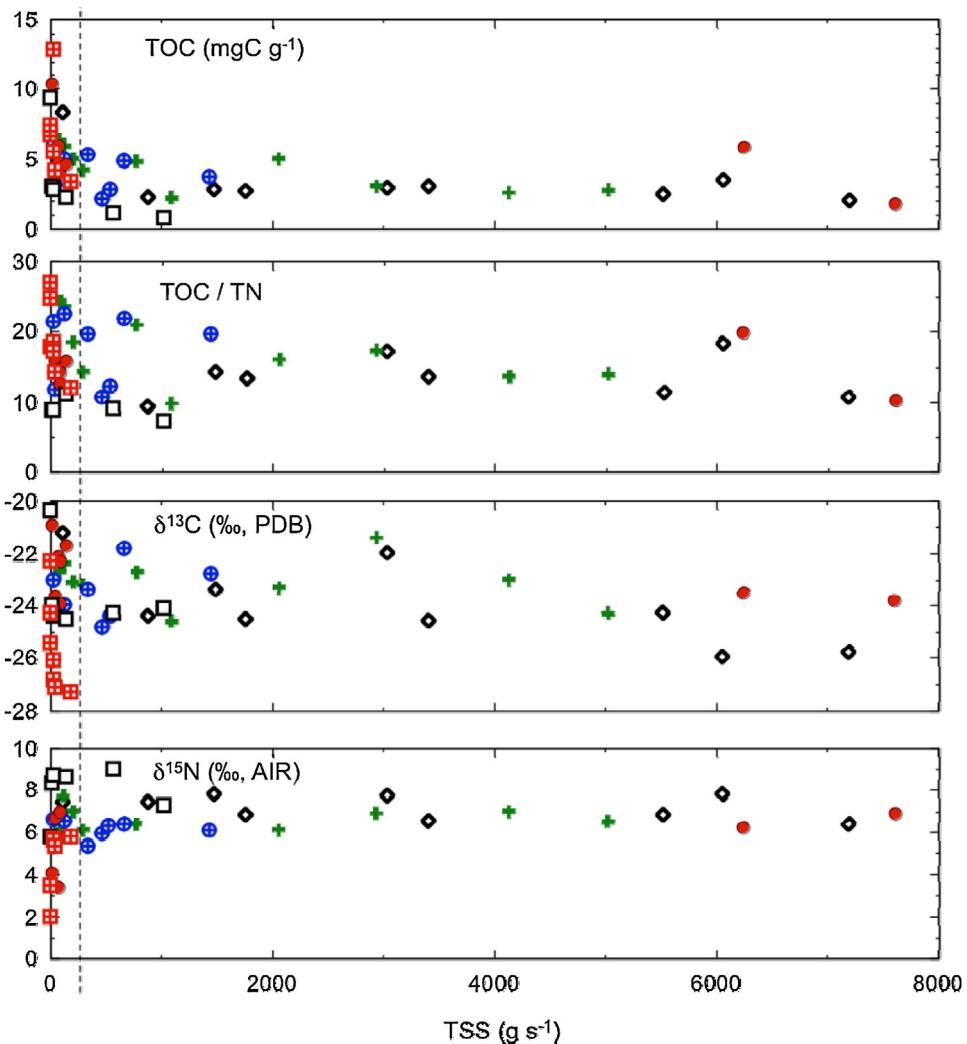
**Fig. 8.** Relations between total suspended sediment (TSS) flux and total organic carbon concentration (TOC), TOC/TN ratio,  $\delta^{13}\text{C}$  and  $\delta^{15}\text{N}$  of particle borne organic matter in TSS loads sampled during the June 2 and 4 floods at 6 stations along the HX continuum (location in Fig. 1). The dashed lines separate TSS with very low sediment yields at ca.  $200 \text{ g s}^{-1}$ . Same legend as in Fig. 7.
