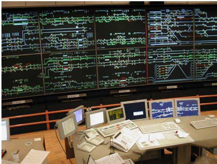
Fig. 1. The information of a very complex process, here in train traffic control in an urban area, forms a pattern that despite its complexity can be perceived and efficiently interpreted by skilled professional traffic controllers.
