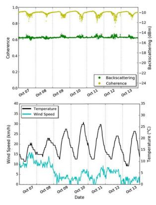
Fig. 10. Focus of (top) RCS and coherence and (bottom) temperature and wind speed, for a week without rain of TS-AUTUMN.
