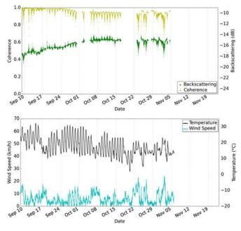
Fig. 7. (Top) RCS and coherence and (bottom) temperature and wind speed for TS-AUTUMN.
