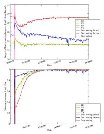
Fig. 6. Evolution of polarimetric (top) RCS and (bottom) coherence of the canopy (3–10-m range) for STS after the watering of the tree. Water was continuously project on the whole tree between the brown and pink vertical lines.
