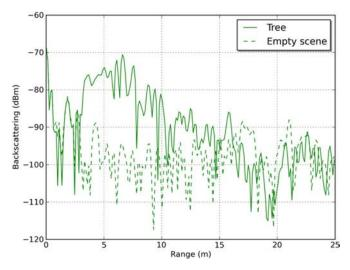
Fig. 3. Impulse response of the scene with and without the tree for polarization HV.
