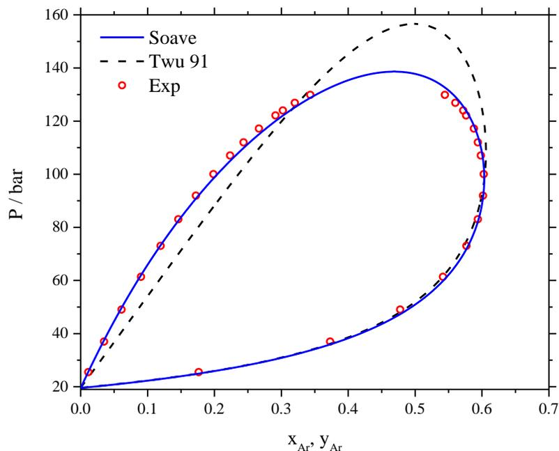
**Figure 1.** Binary phase diagram of the CO<sub>2</sub>-Ar system at 253.1 K calculated with the Peng-Robinson CEoS and two different  $\alpha$ -functions parameterized on subcritical vapor-liquid equilibrium data.
