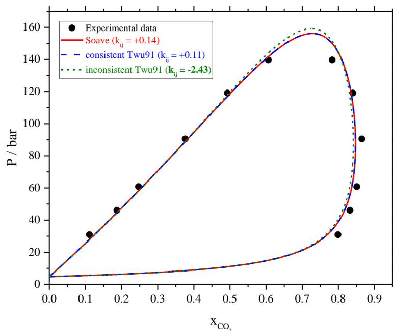
**Figure 13.** Prediction of the CO<sub>2</sub>-n-C<sub>10</sub> phase diagram at 520 K with different  $\alpha$ -functions and classical mixing rules. Red full curve is calculated with the Soave  $\alpha$ -function while blue and green dashed curves are calculated with the Twu91  $\alpha$ -function. Parameters of the  $\alpha$ -function used to calculate the green curve do not satisfy the consistency test while parameters of the blue curve do.
