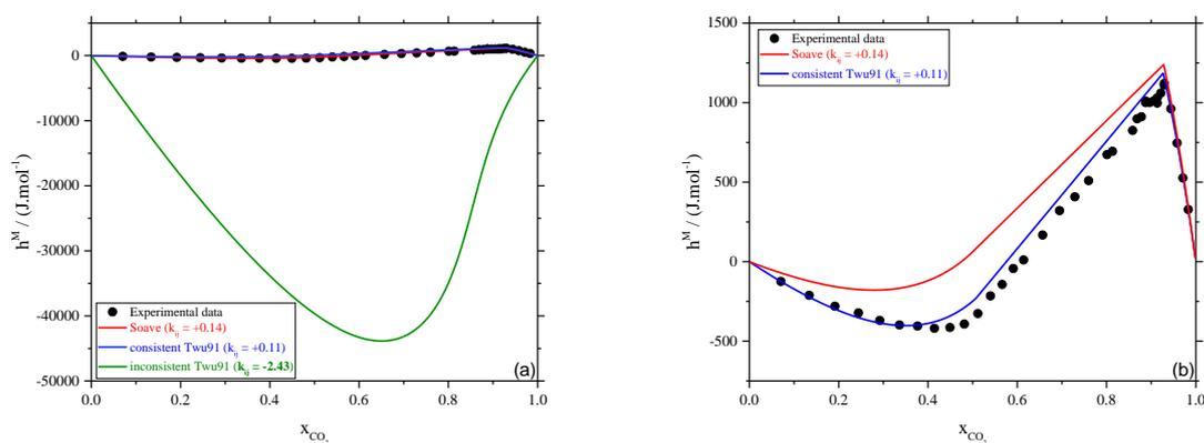
**Figure 14.** Calculation of the mixing enthalpies of the CO<sub>2</sub>-n-C<sub>10</sub> system at 470.11 K and 125 bar.
