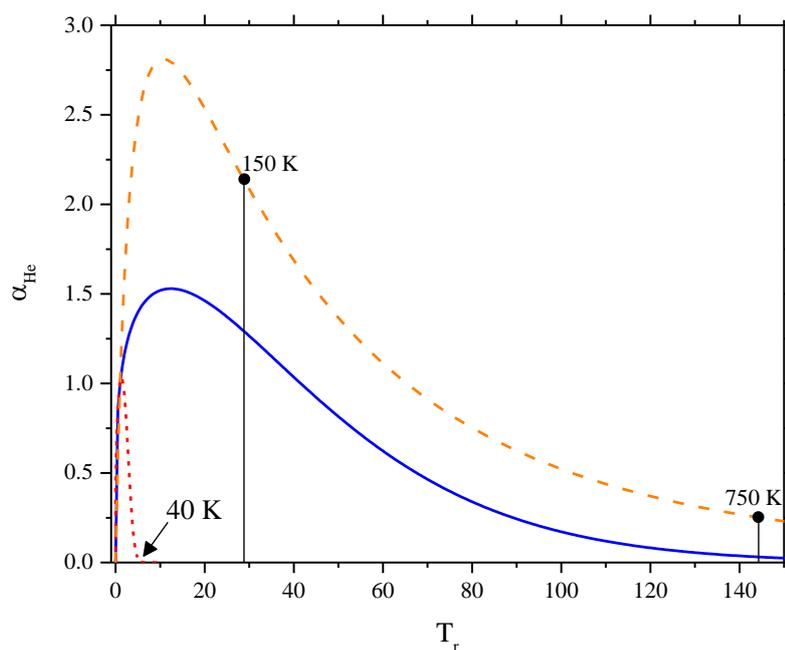
**Figure 18.** Optimized  $\alpha$ -functions of He. Small dashed curve is regressed on subcritical data, large dashed curve is regressed on supercritical data, full curve is regressed on both subcritical and supercritical data.
