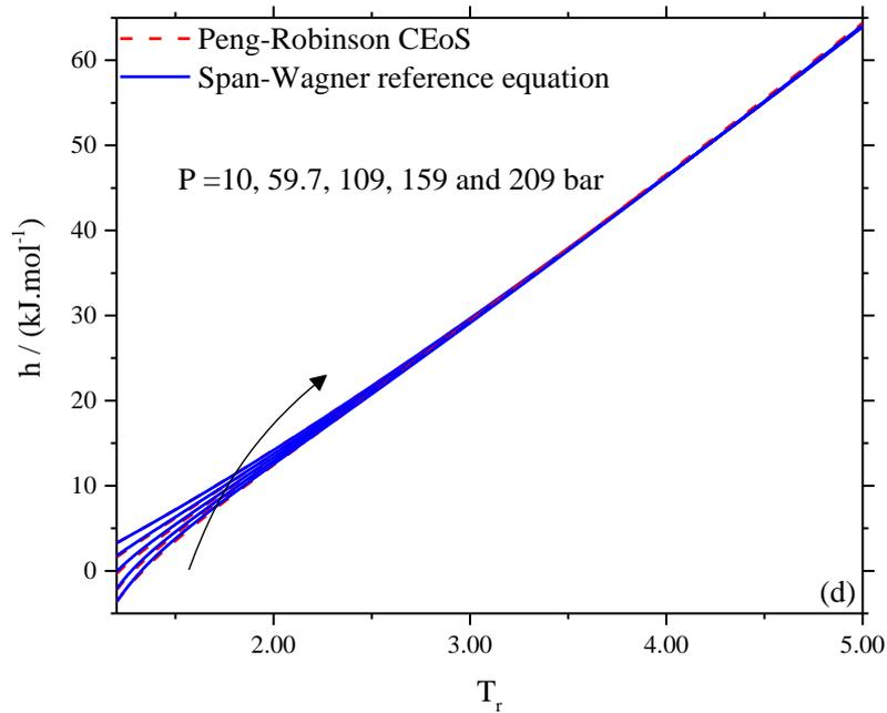
**Figure 11.** Prediction of supercritical  $c_p$  of argon (a) and  $\text{CO}_2$  (b) and prediction of supercritical  $h$  of argon (c) and  $\text{CO}_2$  (d) when constraints  $d^2\alpha/dT^2 > 0$  and  $d^3\alpha/dT^3 < 0$  are both applied.
