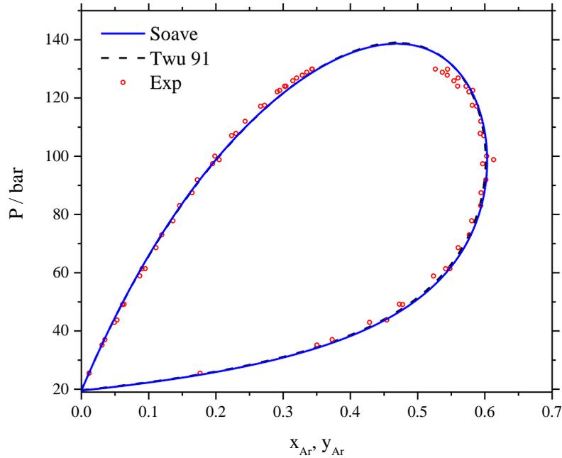
**Figure 12.** Binary phase diagram of the CO<sub>2</sub>-argon system at 253.1 K when constraints  $d^2\alpha/dT^2 > 0$  and  $d^3\alpha/dT^3 < 0$  are simultaneously applied.
