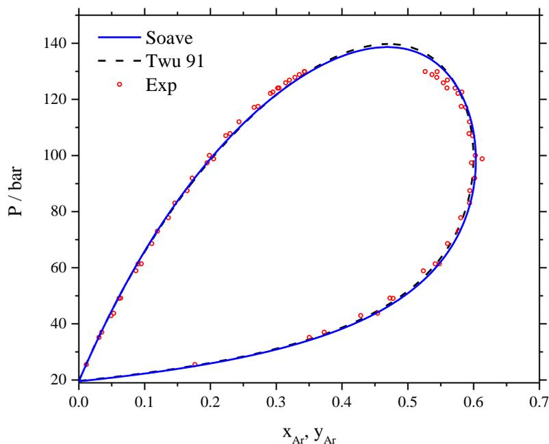
**Figure 7.** Binary phase diagram of the CO<sub>2</sub>-Ar system at 253.1 K when the convexity constraint is enforced ( $d^2\alpha/dT^2 > 0$ ).
