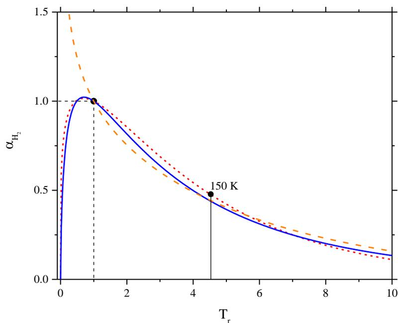
**Figure 19.** Optimized  $\alpha$ -functions of H<sub>2</sub>. Small dashed curve is regressed on subcritical data, large dashed curve is regressed on supercritical data, full curve is regressed on both subcritical and supercritical data.
