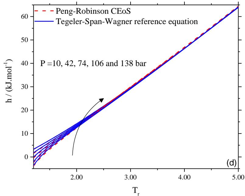
**Figure 8.** Prediction of supercritical  $c_p$  of argon (a) and CO<sub>2</sub> (b) and prediction of supercritical  $h$  of argon (c) and CO<sub>2</sub> (d) when convexity constraint ( $d^2\alpha/dT^2 > 0$ ) only is applied.
