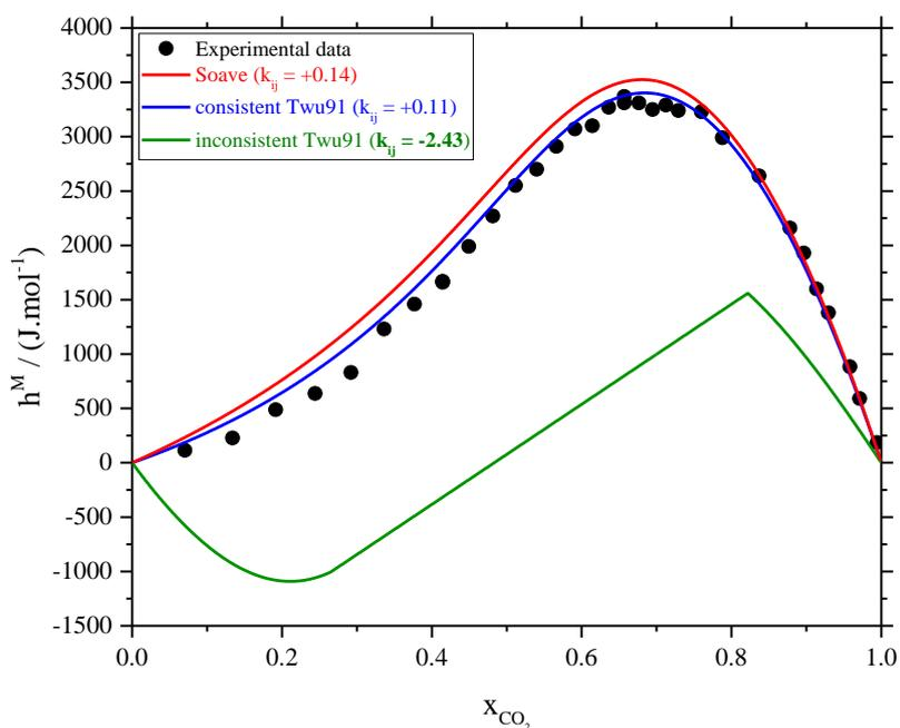
**Figure 15.** Calculation of the mixing enthalpies of the CO<sub>2</sub>–n-C<sub>10</sub> system at 573.11 K and 125 bar.
