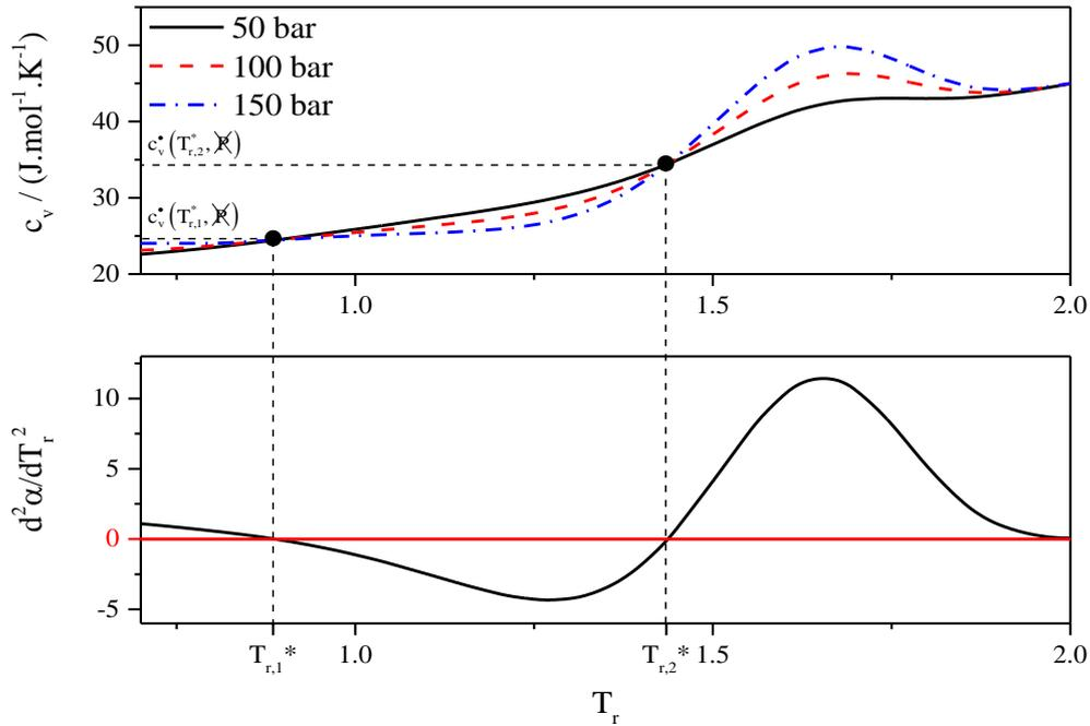
**Figure 4.** Illustration of the unphysical isobars crossing when the second derivative of an  $\alpha$ -function cancels – case of CO<sub>2</sub>.
