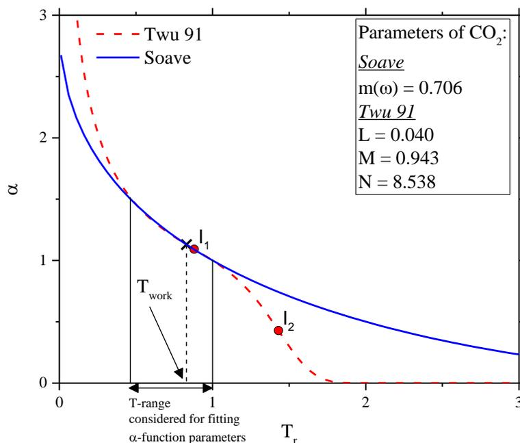
**Figure 2.**  $\alpha$ -curves of CO<sub>2</sub> parameterized on subcritical vapor-liquid equilibrium data.
