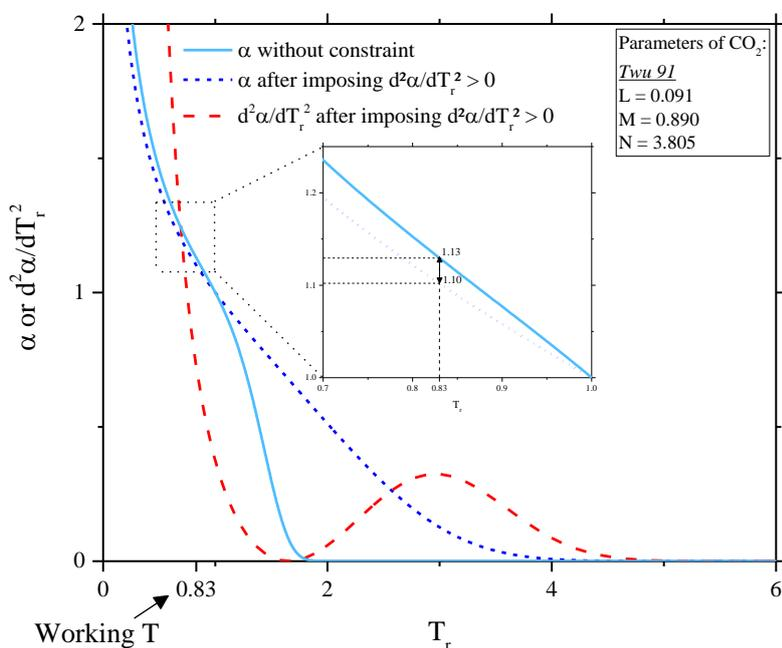
**Figure 6.**  $\alpha$ -function of pure CO<sub>2</sub> and its second derivative when the convexity constraint is enforced.
