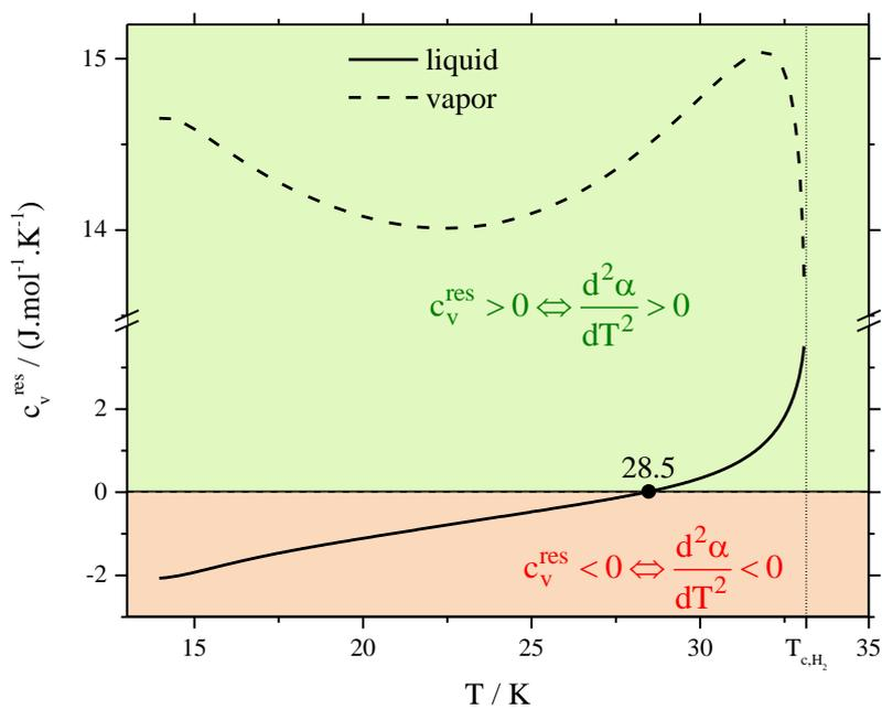
**Figure 16.** Residual heat capacities of vapor and liquid phases of saturated H<sub>2</sub>.
