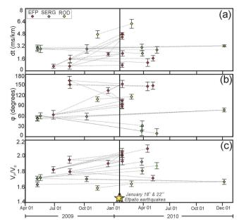
**Figure 6.** Diagrams showing the variation of (a) the measured shear wave time-delays dt, (b) fast polarization directions  $\varphi$  and (c)  $V_P/V_S$  ratios from 2009 January to 2010 December for event doublets. The time-delays were normalized according to the hypocentral distances. Black vertical bars represent measurement errors.
