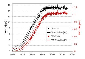
**Figure 1.** Mixing ratios of CFC-114 and CFC-114a as measured in air samples collected at Cape Grim, Australia, between 1978 and 2014 (diamonds) and derived from two Antarctic firn air profiles (lines). Uncertainties are  $1\sigma$  standard deviations for Cape Grim data and a combination of the former and a firn modelling uncertainty for the latter (shown as dashed lines, see text for further details).
