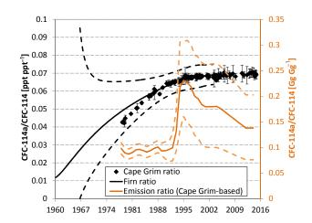
**Figure 2.** CFC-114a / CFC-114 ratio of mixing ratios at Cape Grim (left axis, black diamonds) and derived from Antarctic firn (left axis, black line), as well as the ratio of their emissions derived from these observations (right axis, orange line). Uncertainties of those ratios are calculated from the uncertainties of mixing ratios (Fig. 1) and emissions (Fig. 3) and using the equation for combining errors in quotients.
