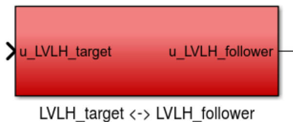
Figure 8: Change the coordinate frame of the input from leader LVLH to follower LVLH.
