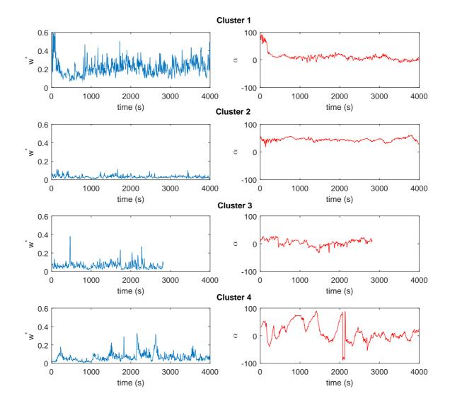
FIG. 6: Examples of signals analysed to each cluster (from top to bottom). The wind vertical velocity fluctuations  $w^*$  (left) and the angle  $\alpha$  as a function of time.
