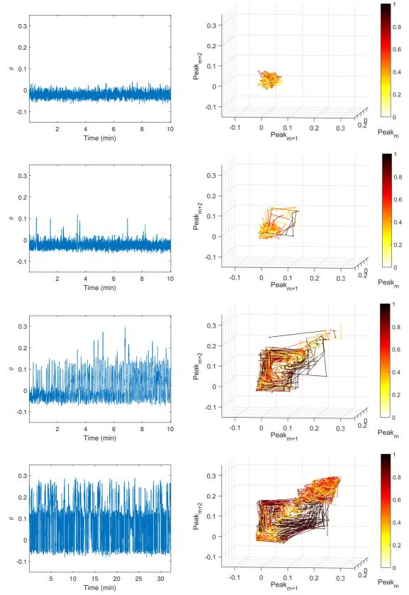
FIG. 4: Left panels: time series of the reduced rotation frequency  $\theta$ . Right panels: the attractor representation obtained via a three dimensional embedding of  $\theta$ . From top to bottom  $\gamma$  is increased from 0 to 0.06. The color represents the stability of the points of the attractor measured by  $\Upsilon$ .
