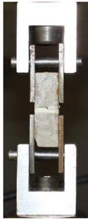
Figure 2: Tensile test on the concrete sample
