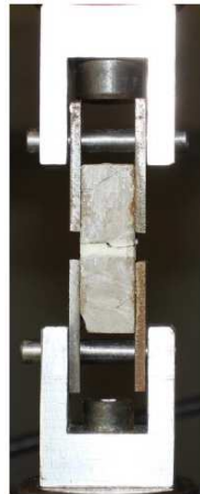
Figure 2: Tensile test on the concrete sample
