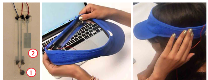
Figure 6. A Stretchi integrated into a stretchable headband. The Stretchi includes a (1) rigid vibration motor that sends notifications to the wearer and a (2) stretchable touch sensor to support touch interaction.
