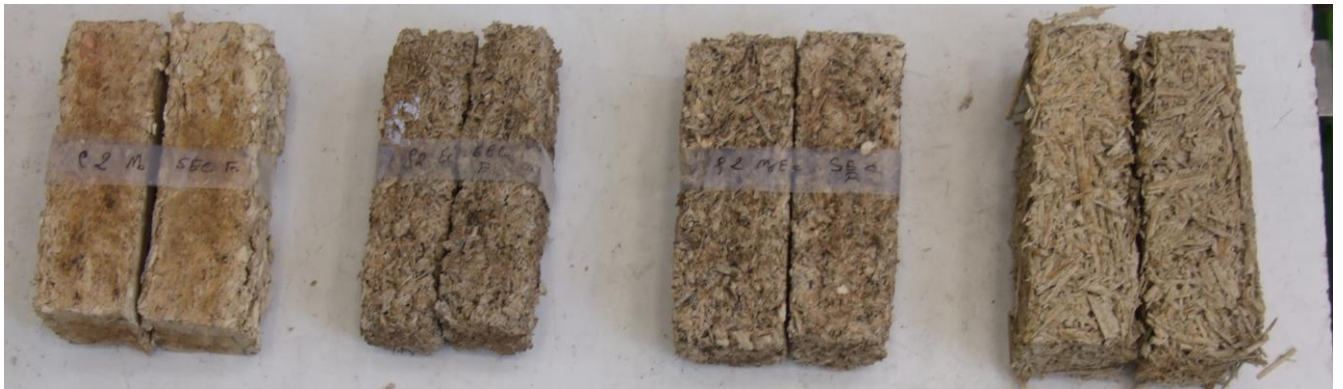
Fig 1. Samples for thermal conductivity measurements, from left to right: clay-sunflower pith, clay-sunflower bark, clay-sunflower bark and pith and clay rape-straw
