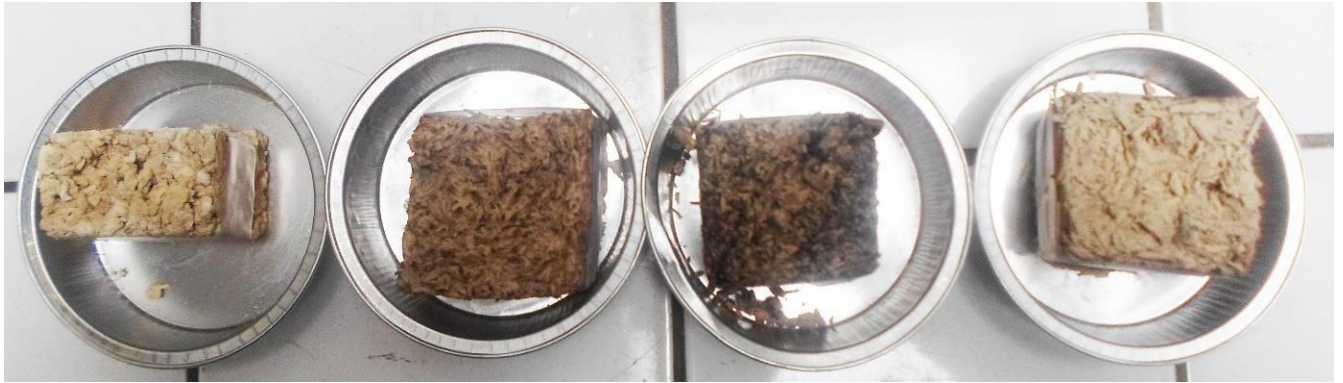
Fig 1. Samples for sorption/desorption measurements, from left to right: clay-sunflower pith, clay-sunflower bark, clay-sunflower bark and pith and clay rape-straw
