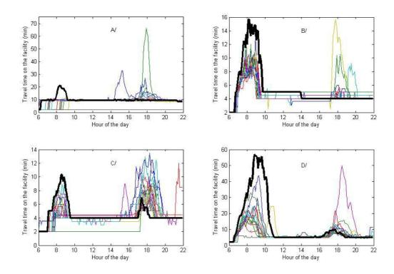
**Figure 3:** Travel times for the four chosen facilities for the 19 studied days. We can notice that D/ is the most congested facility in morning peak, that both morning and evening peaks create problems for route C/ which is a ring road. A/ is a facility highly used by trucks, and is less exposed to morning or evening congestion, except when incidents occur. The bold line corresponds to the results obtained the  $4^{\text{th}}$  of October, 2005.
