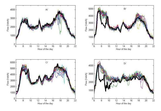
**Figure 4:** Measured flows for the four chosen facilities during the 19 studied days. The bold line corresponds to the results obtained the 4<sup>th</sup> of October, 2005.
