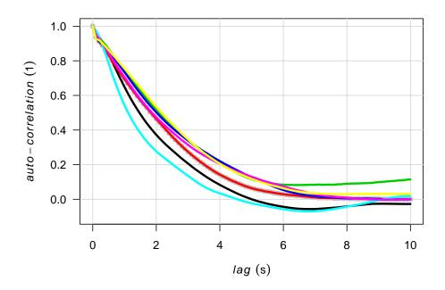
FIGURE 3 Auto-correlation function of the acceleration of seven vehicles, again taken from the simTD data.
