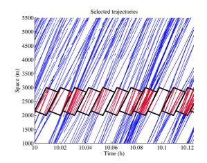
(b) The trajectories in x-t plane of the vehicles in all lanes. A parallelogram is used as aggregation interval: in this 7,5 minute period 11 different aggregation areas are identified. Note that there are gaps and periods with vehicles with shorter headways, and that borders of the integration area is well aligned with the borders between traffic operations.
