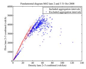
(a) Fundamental diagram in flow-density plane.
