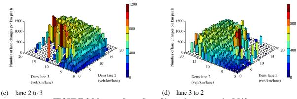
FIGURE 8 Measured number of lane changes on the M42
