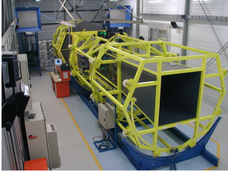
FIGURE 2. Side view schematic representation and two pictures of the wind tunnel specifically designed for the study of thermally stratified shear layers. Left picture is a wind tunnel overview. Right picture focuses on the test section with the splitter plate and a laser-sheet flow visualization of the mixing layer.
