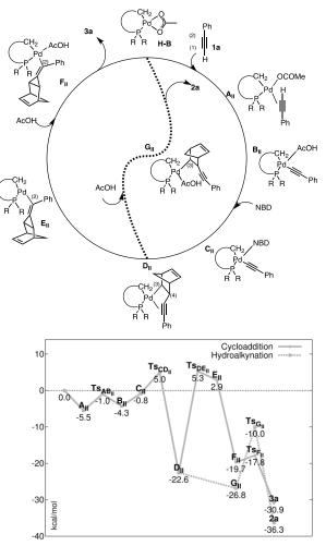
Scheme 4. Catalytic cycles for either the hydroalkynation or the formal [2+1] cycloaddition of NBD and 1a (2a and 3a, Scheme 1) with the H-B catalyst, according to approach II (1a coordinates the Pd *cis* to the phosphine). The catalyst is schematically sketched. The R substituent is o-Tol. The computed energetic profiles (M06/def2-SVP//M06/def2-TZVP, ZPE at the optimizing level) are reported below. Energies are relative to the separated species (catalyst + reactant).
