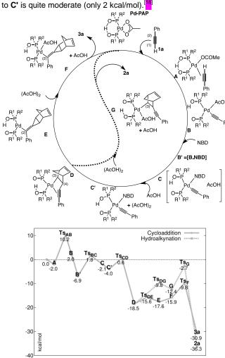
**Scheme 5.** Catalytic cycles for either the hydroalkynation or the formal [2+1] cycloaddition of NBD and **1a** (**2a** and **3a**, Scheme 1) with **Pd-PAP** catalyst ( $R^1 = Ph$ ,  $R^2 = tBu$ ). The computed energetic profiles (M06/def2-SVP//M06/def2-TZVP, ZPE at the optimizing level) are reported below. Energies are relative to the separated species (catalyst + reactant).
