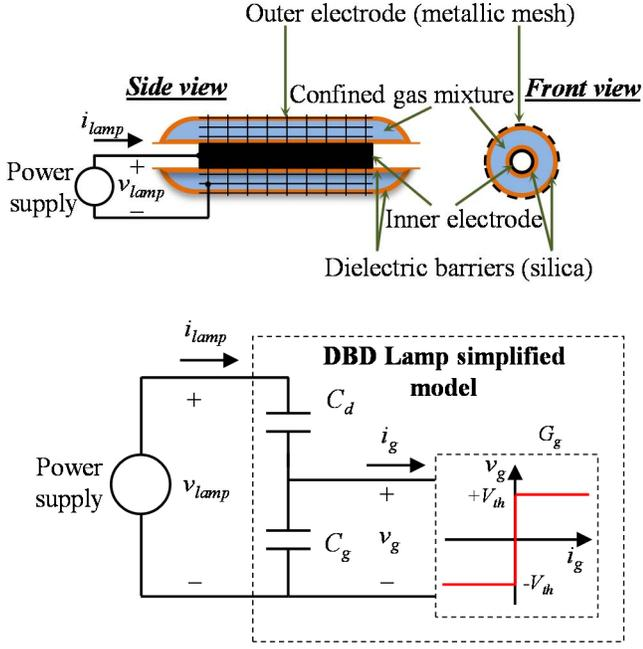
Fig. 1. DBD excitlamp. Physical structure (top) and equivalent electric model (bottom).
