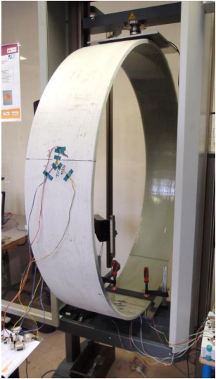
Figure 2. Radial compression set-up.
