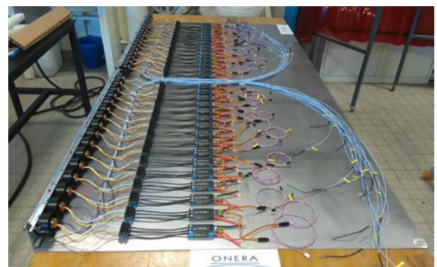
Fig. 15 – Ground test bench for propulsion architecture validation
