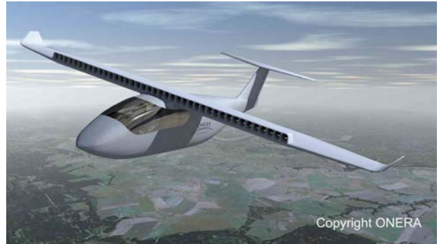
Fig. 5: High-wing concept-plane with distributed EDF along the wing leading edge
