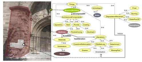
Fig. 3. Domain Ontology sample dedicated to masonry building alteration monitoring: alveolization example
